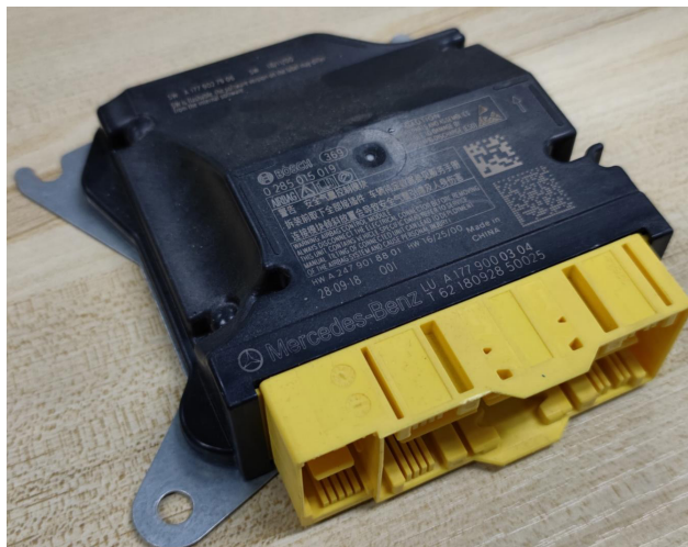
Figure 9.3: Airbag control module
